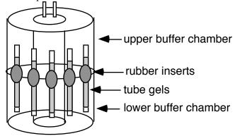
If less than 12 tube gels are going to be run, fill the remaining rubber inserts with "blanks"-- unusable poured gels or empty tubes (which must be placed above the level of the upper buffer-approx. 1 inch from the top). It is important that *all 12* rubber inserts contain a tube to ensure that no upper buffer can leak into the lower chamber.
